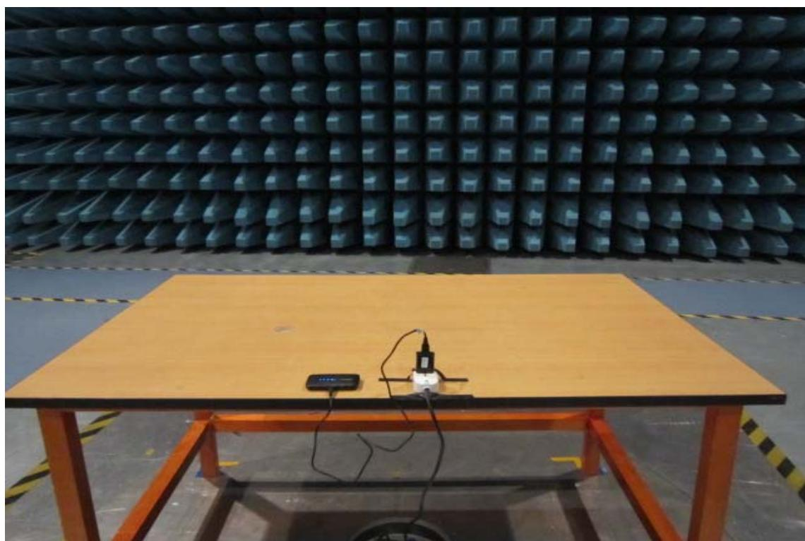
FCC Part15C Radiated Emission above 1GHz
