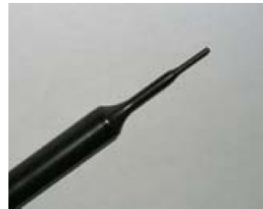
Picture C.2 Near-field Probe
