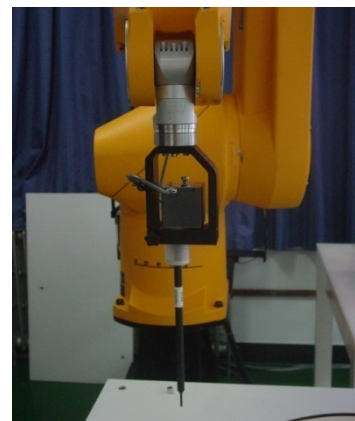
Picture C.3 E-field Probe
