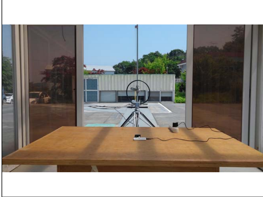
Radiated Emission (below 30 MHz_with Load, Pad type)
