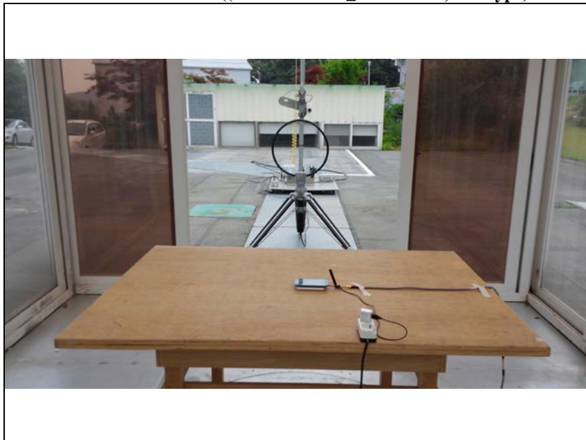
Radiated Emission ((below 30 MHz_with Phone, Pad type)
