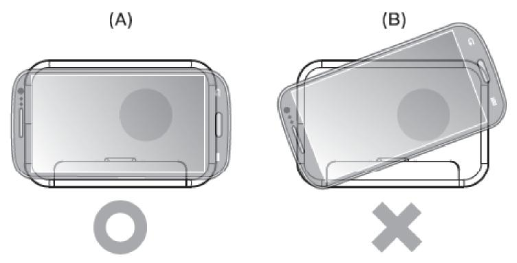
The transmitting coil is located in the area of as shown in the pictures above. The coil of the charger and it of the device have to be aligned each other to make wireless charging work properly as shown in the picture (A).
