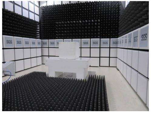
**Conducted Peak Output power Test Setup**
