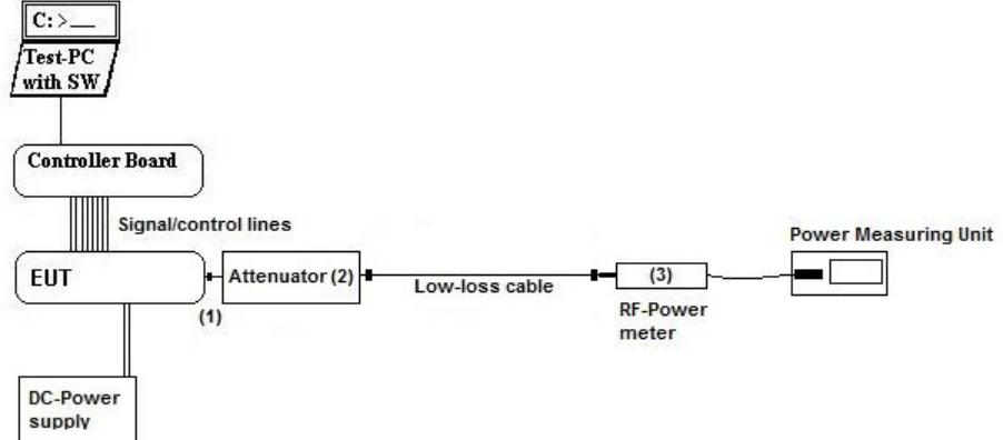
**Testing method:** ANSI C63.10:2013, KDB 558074 D01 DTS Meas. Guidance v05r02
