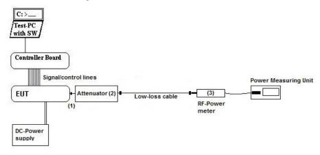
**Testing method:** ANSI C63.10:2013, KDB 558074 D01 DTS Meas.Guidance v04
