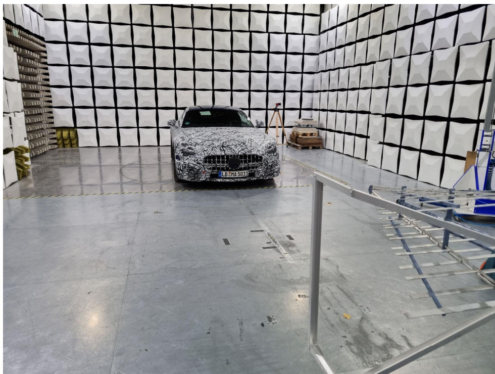
Fig. 5: Set up with EUT for test without absorbers at a car (C192 AMG GT)
