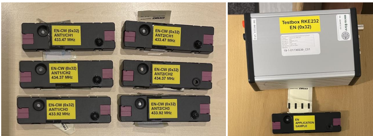
Fig. 5: Photos of the CW modules (on the left) and system providing the modulated signal (on the right) for EU.
