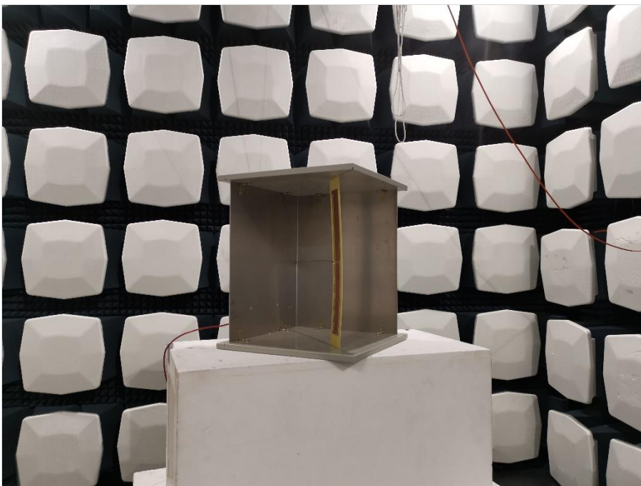
Photograph 2: Close view of the test Setup in the fully anechoic chamber. Radiated interference field strength. EUT is at standing position.
