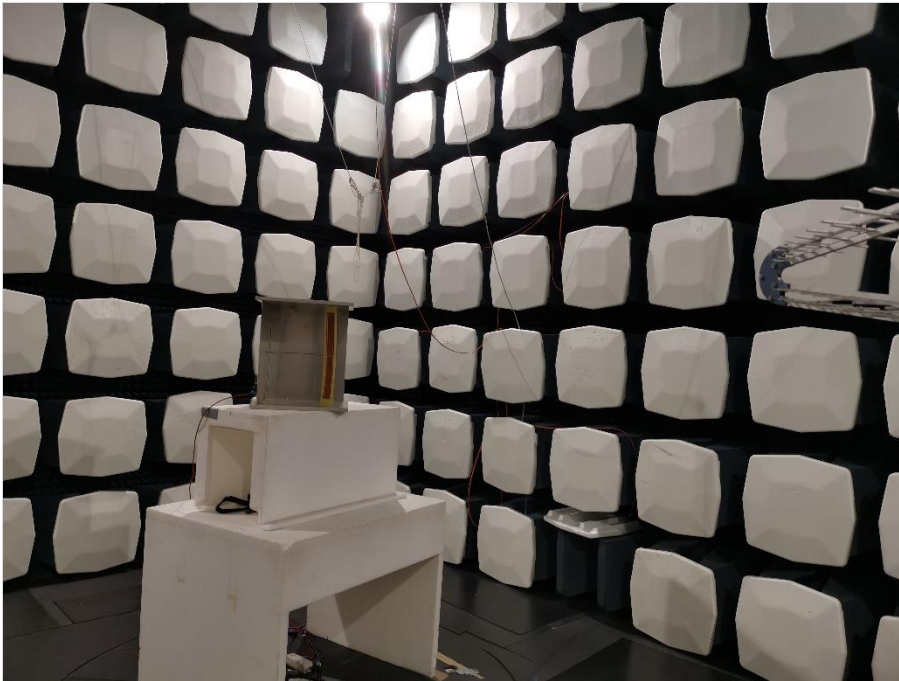
Photograph 1: Overview of the test Setup in the fully anechoic chamber. Radiated interference field strength. EUT is at standing position.
