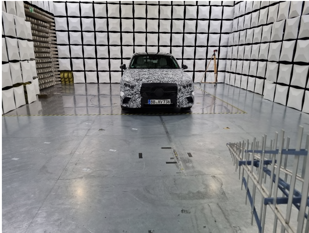
Fig. 5: Set up with EUT for test without absorbers at a car (Mercedes Benz (S214) E class station wagon)
