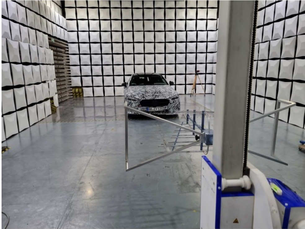
Fig. 5: Set up with EUT for test without absorbers at a car (C-Class (C236))
