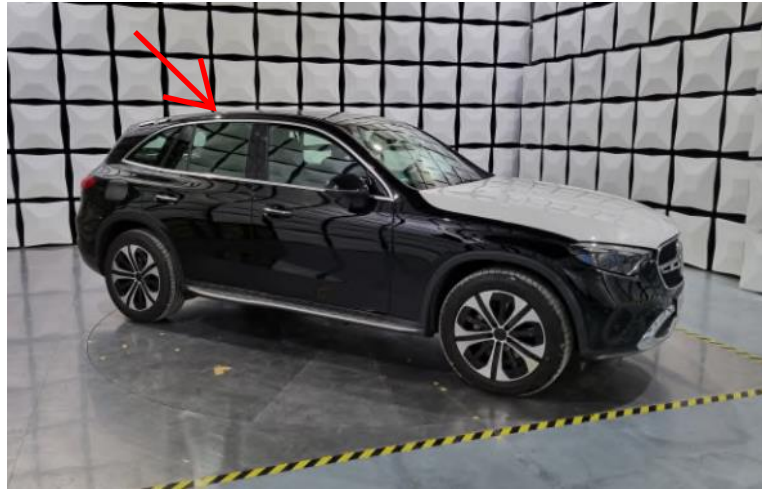
Mounting position of the Telematics Module
