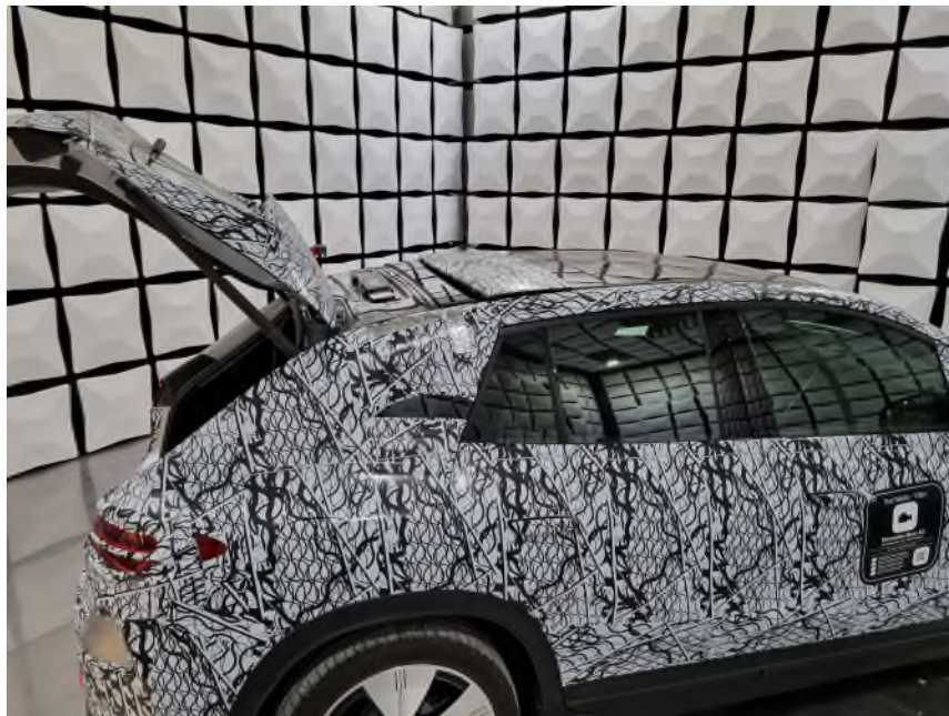
Fig. 6: EUT support details: set up when measuring the real antenna installed at the car (with cover removed)
