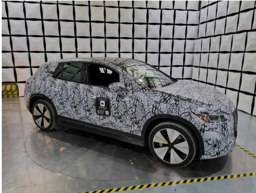
Fig. 5: Set up with EUT for test without absorbers at a car (EQE SUV (X294))
