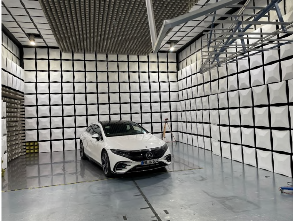
Fig. 5: Set up with EUT for test without absorbers at a car (EQS (V297)).
