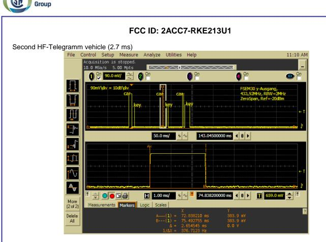
100 ms time window in the range of the first HF-Telegramm Both Marker show the 100 ms time window.
