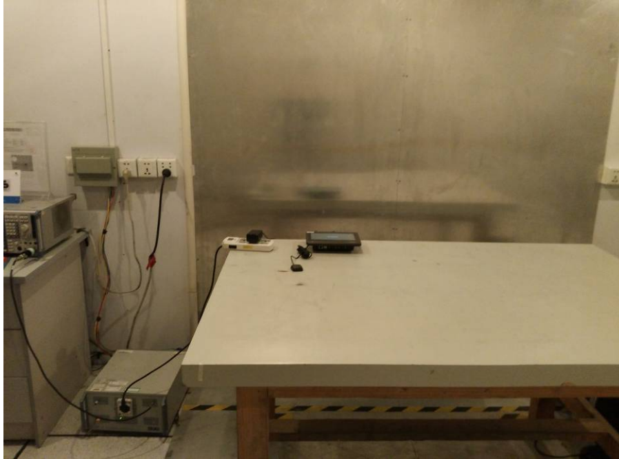
CONDUCTED EMISSION TEST
