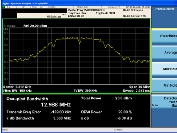
(802.11b) 6dB Bandwidth plot on channel 6
