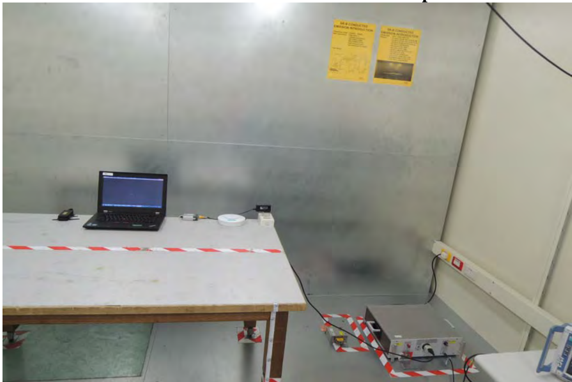
AC Power-line Conducted Emission Set up Photo
