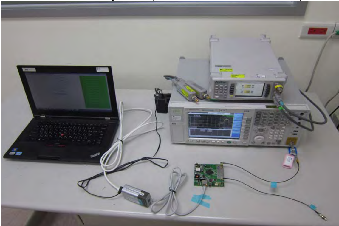
Conducted Setup Photo (Measurement at Antenna Port)
