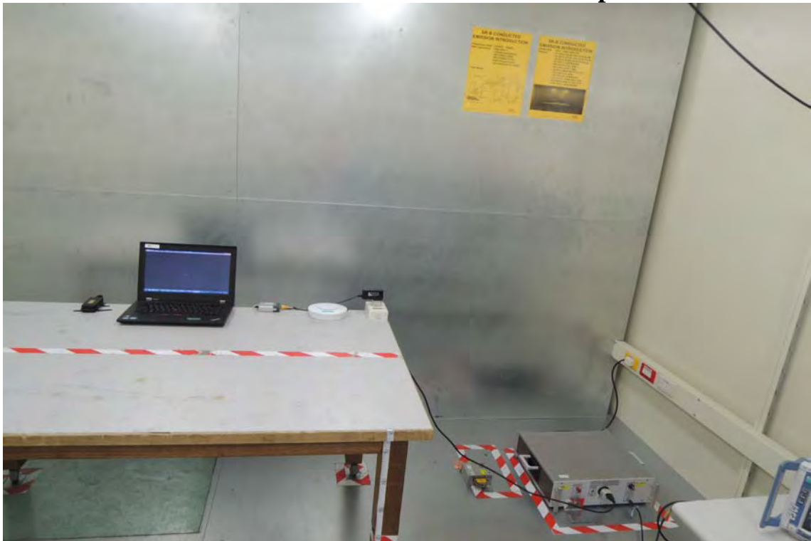
AC Power-line Conducted Emission Set up Photo
