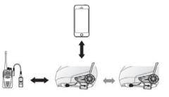
Frontmost and backmost members of the group (A and F) can connect with any two devices of mobile phones, GPS or adaptors apart from connecting with one group
