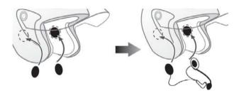
Open the lining of helmet (at ear's position), clean the EPS surface and affix the VELCRO on with the rough surface
