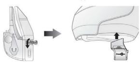
Loosen the screw on the back of universal helmet clamp with the provided screw driver
