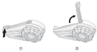
Push the antenna slightly along the arrow direction in figure ① and it will open automatically along the arrow direction in figure ②
