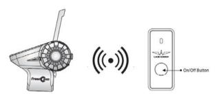
Step 1: Ensure T-Rex is off and within 1 m visible range of the device to be paired.
