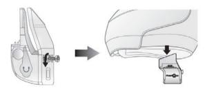
Loosen the screw on the back of universal clamp with the provided screw driver  Remove the clamp from helmet (along the arrow direction in figure)
