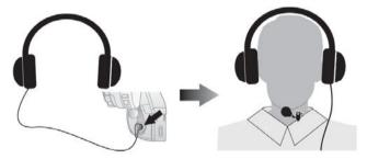
(3) Insert the normal Ø3.5mm headphone plug into the Ø3.5mm jack on universal clamp
