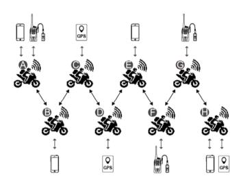
1500 m intercom range, chain-shaped connection with unlimited links, preferably 8 links; can be connected with multiple devices (mobile phones, GPS and adaptors).
