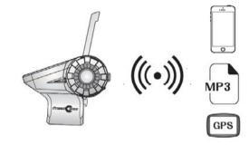
Step 1: Ensure T-Rex is off and within 1 m visible range of the device to be paired.
