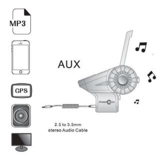
(3) Audio in Mp3, mobile phone, GPS, stereo and PC that are without Bluetooth can be imported into the Bluetooth device through stereo audio cable. (usable when the Bluetooth
