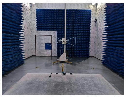
RADIATED EMISSION TEST SETUP ABOVE 1GHz
