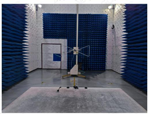
RADIATED EMISSION TEST SETUP ABOVE 1GHz
