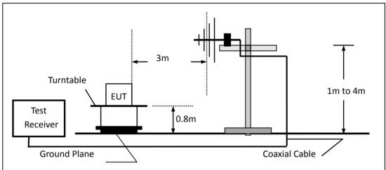
(c) For radiated emissions above 1000MHz
