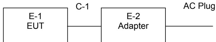
Radiated Spurious Emission Test
