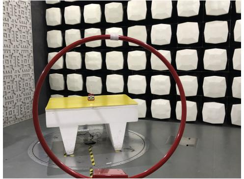
1.2 Radiated Emissions Test Setup
