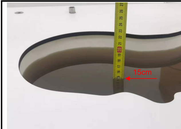
Figure 12-1 Liquid depth in the Head Phantom
