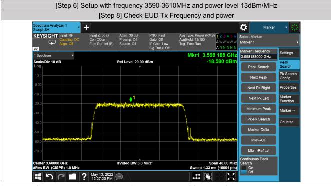
EIRP PSD=-19.580-0.13+5=-14.71dBm/MHz, attenuation of Cable and Splitter is 5dB, Antenna gain is - 0.13dBi.
