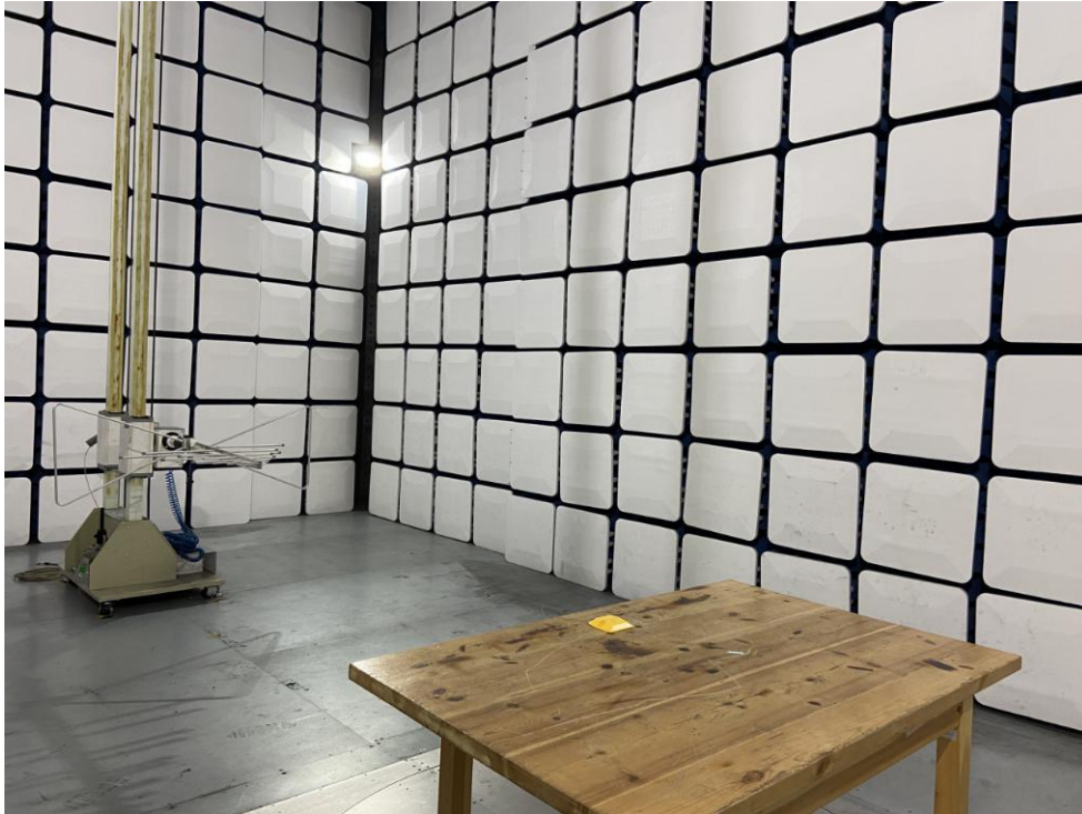
Photo of Radiation Emission Test
