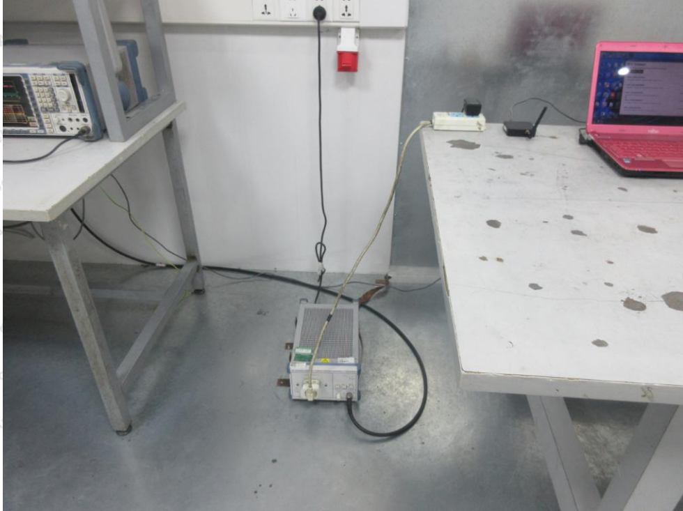
Photo of Power Line Conducted Emission Test
