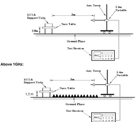
The radiated emission tests were performed in the 3 meters chamber test site, using the setup accordance with the ANSI C63.10-2013. The specification used was the FCC 15.209, and FCC 15.247 limits.
