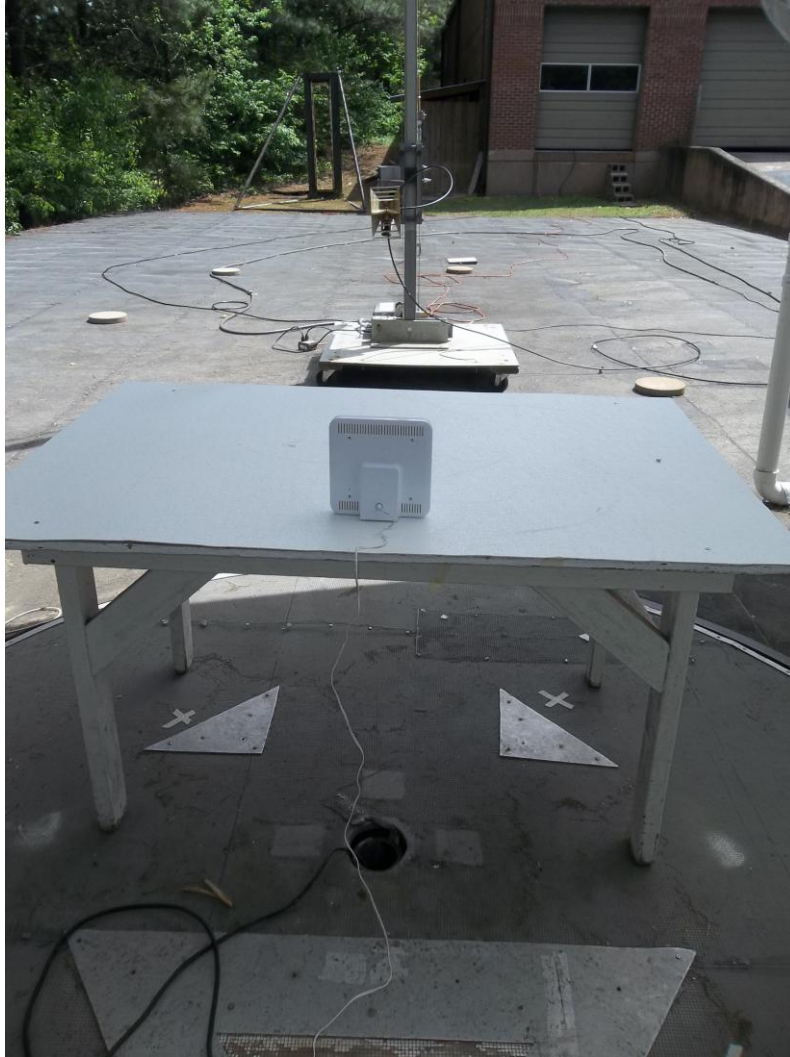
Figure 3. Radiated Emissions Test Set Up (Above 1 GHz)
