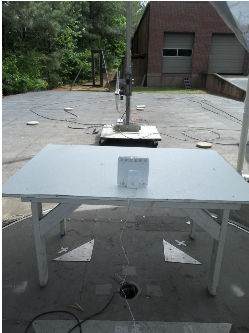
Figure 5. Radiated Emissions Test Setup (200-1000 MHz)
