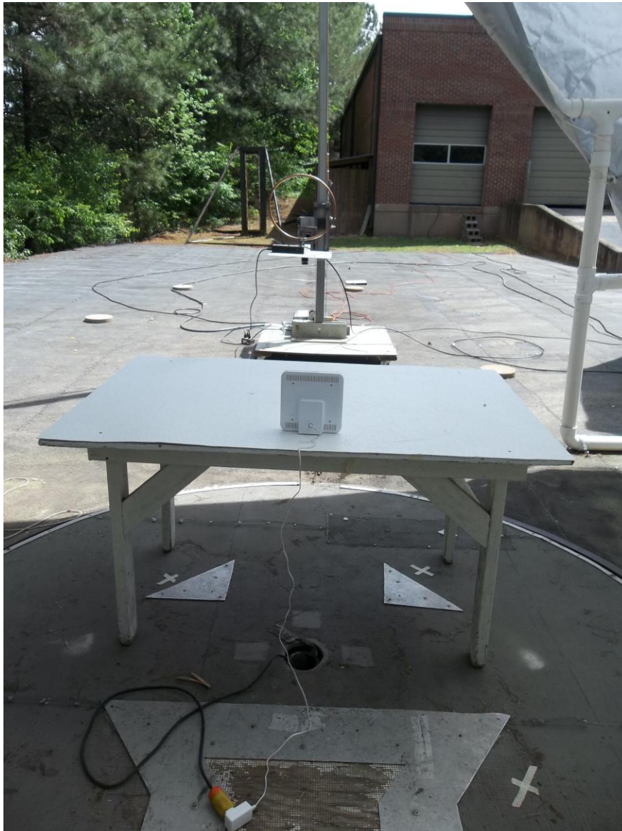
Figure 6. Radiated Emissions Test Setup (Below 30 MHz)
