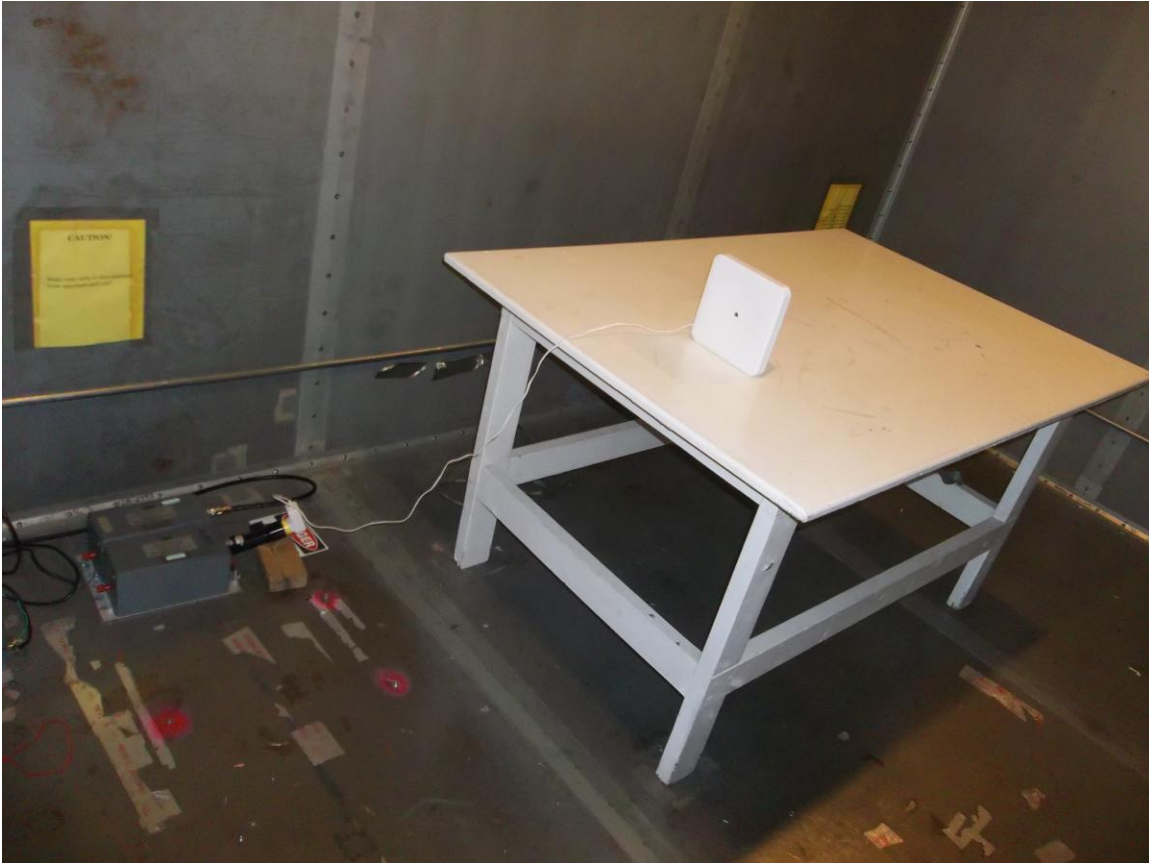
Figure 1. Powerline Conducted Emissions Test Setup
