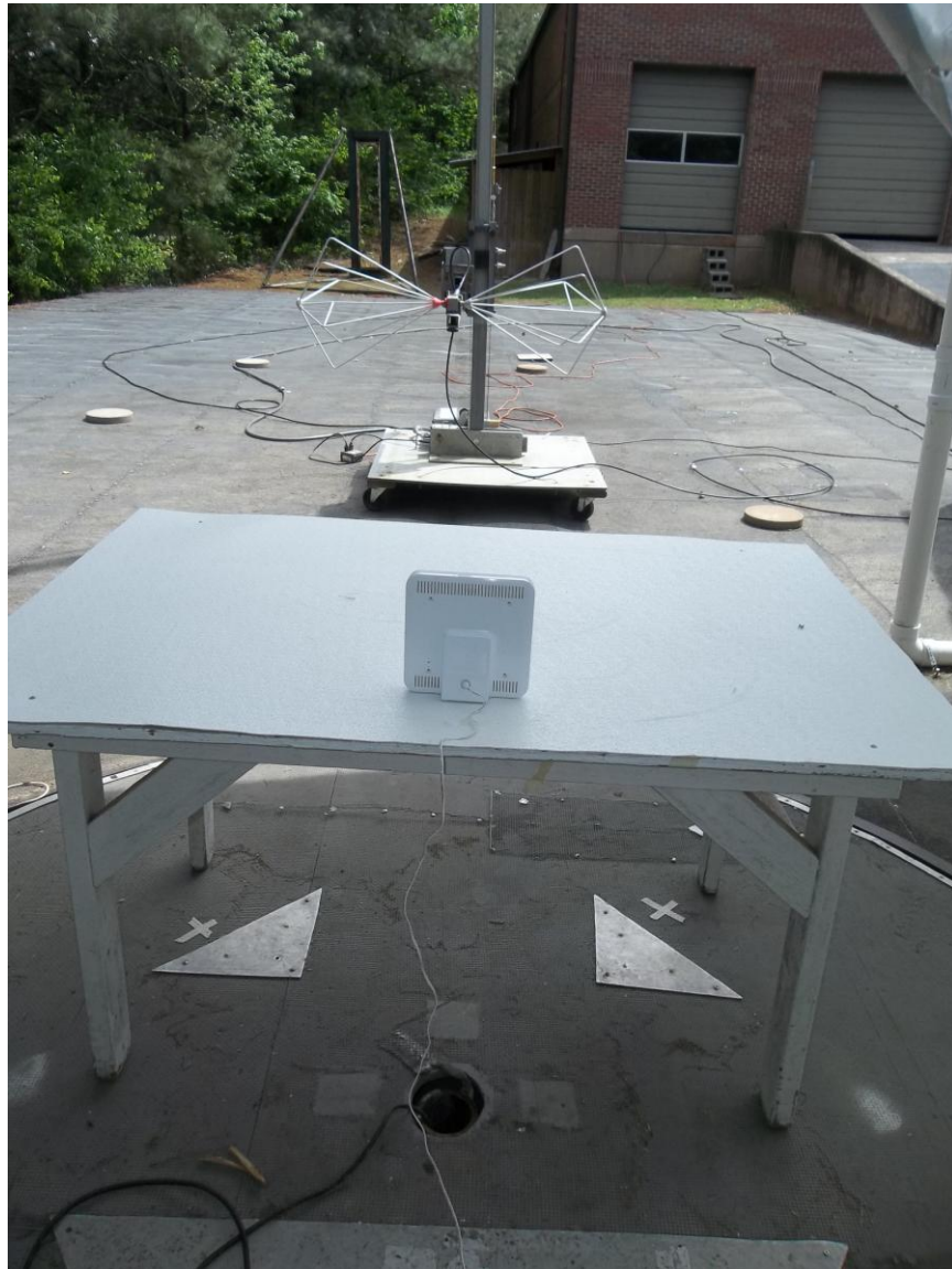
Figure 4. Radiated Emissions Test Setup (30-200 MHz)
