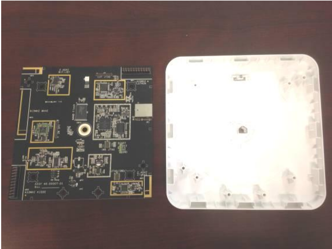
Figure 2. PCB Removed from the Enclosure
