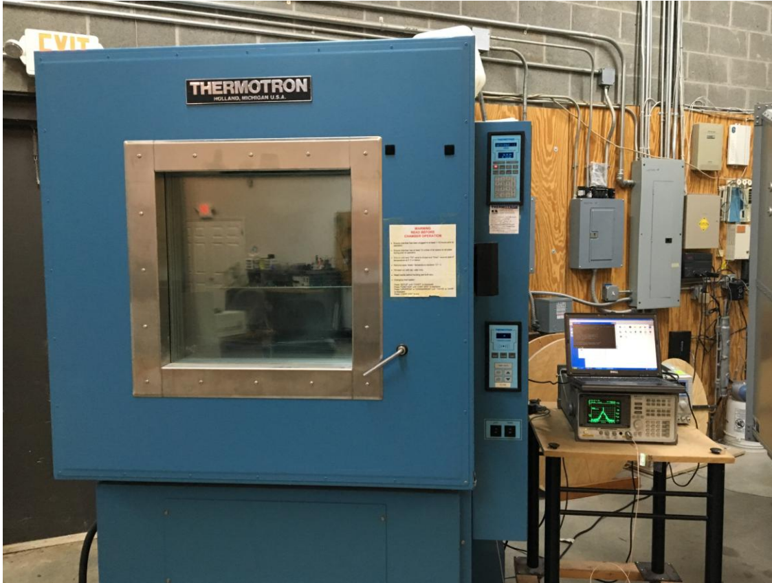
Figure 9. Extreme Temperature and Frequency Stability Test Setup
