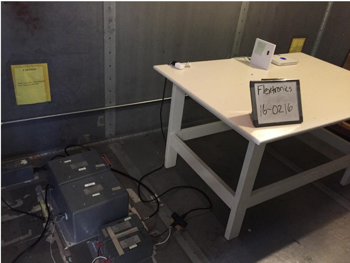
Figure 1. Powerline Conducted Emissions Test Setup for All Radios (all radios ON and exercising)
