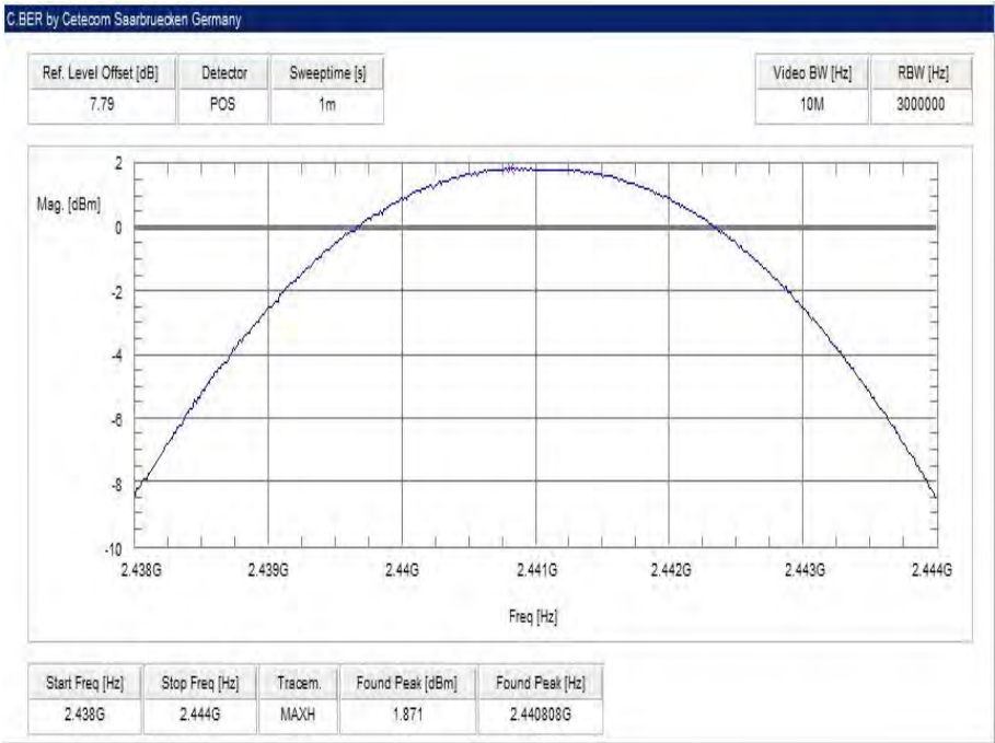
Plot 5: middle channel – 2441 MHz, Pi / DQPSK modulation
