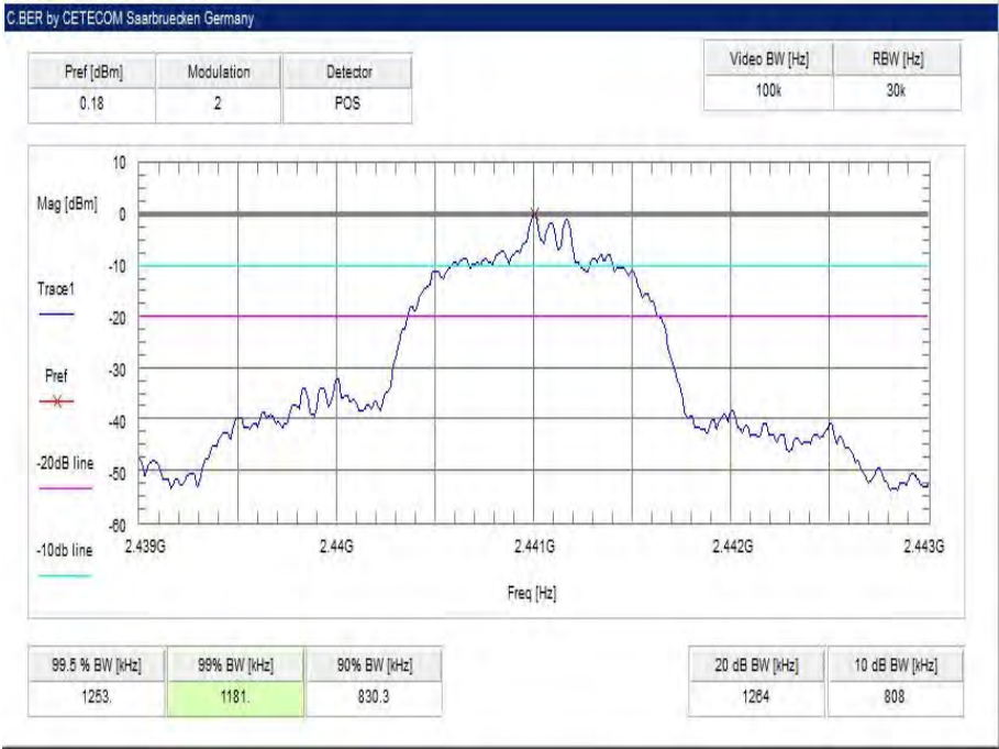
Plot 8: middle channel – 2441 MHz, 8 DPSK modulation
