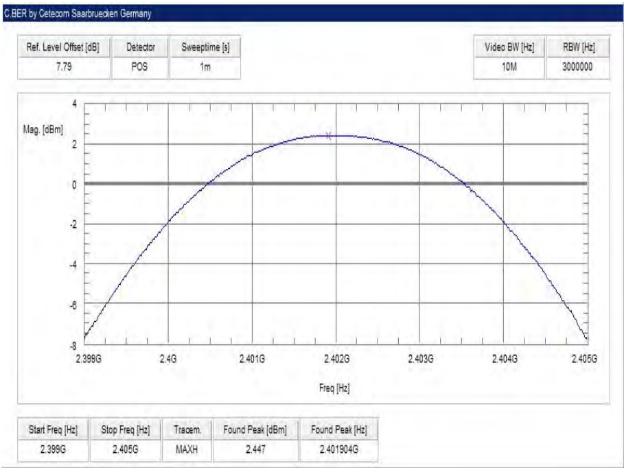
Plot 4: lowest channel – 2402 MHz, Pi / DQPSK modulation
