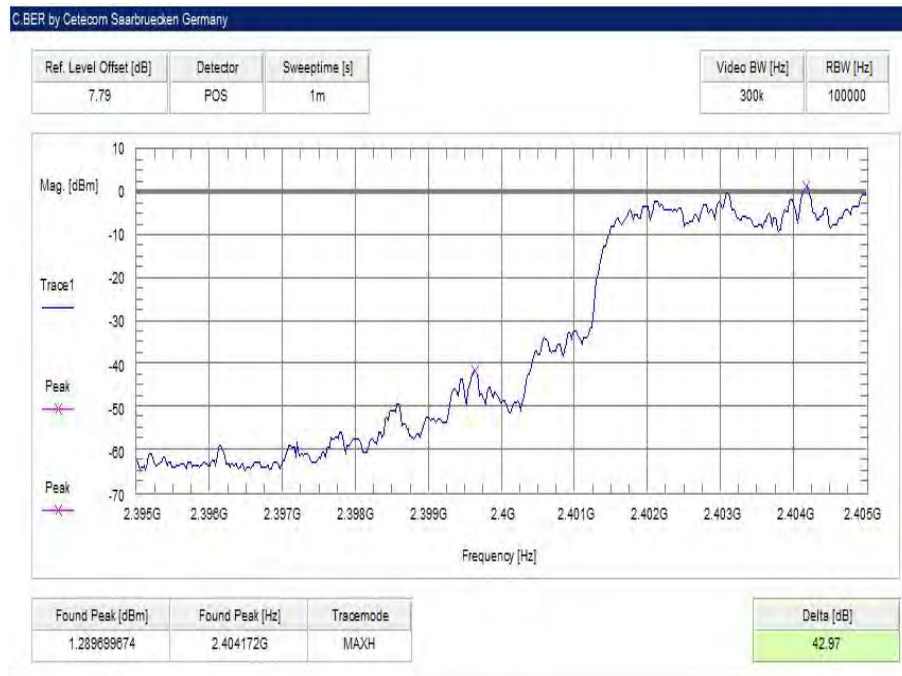
Plot 9: Lower band edge – hopping on, 8DPSK modulation
