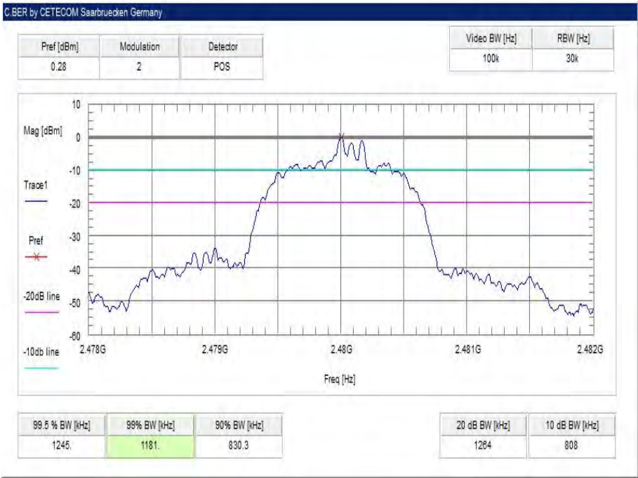
Plot 9: highest channel – 2480 MHz, 8 DPSK modulation
