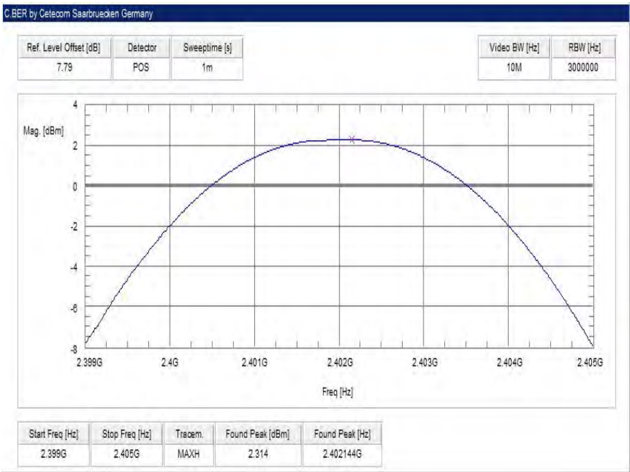
Plot 1: lowest channel – 2402 MHz, GFSK modulation
