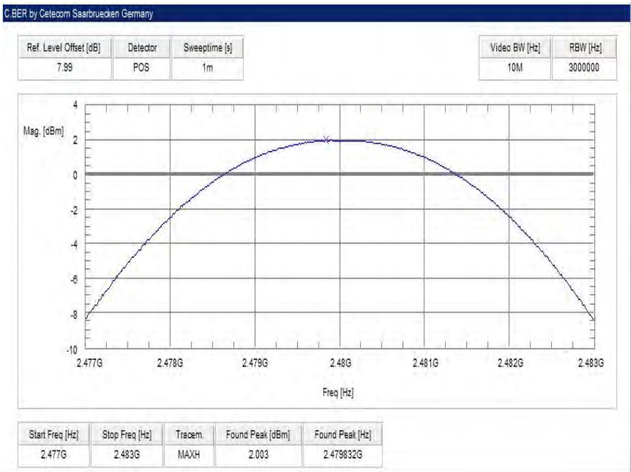
Plot 6: highest channel – 2480 MHz, Pi / DQPSK modulation
