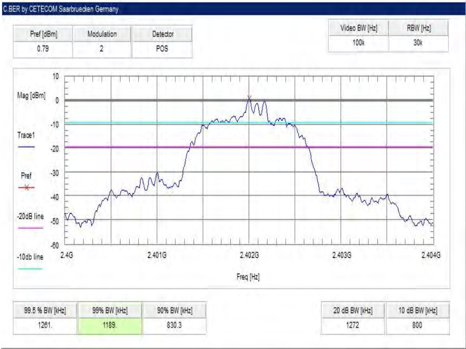
Plot 7: lowest channel – 2402 MHz, 8 DPSK modulation
