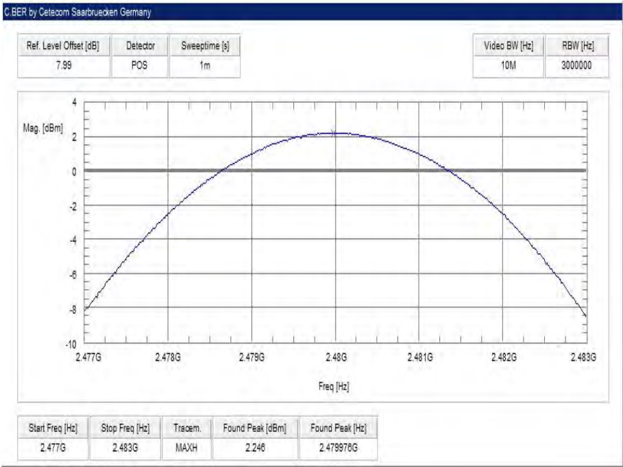
Plot 9: highest channel – 2480 MHz, 8 DPSK modulation
