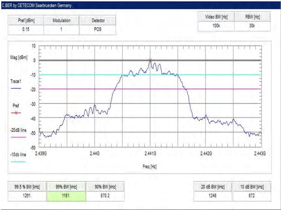
Plot 5: middle channel – 2441 MHz, Pi / DQPSK modulation
