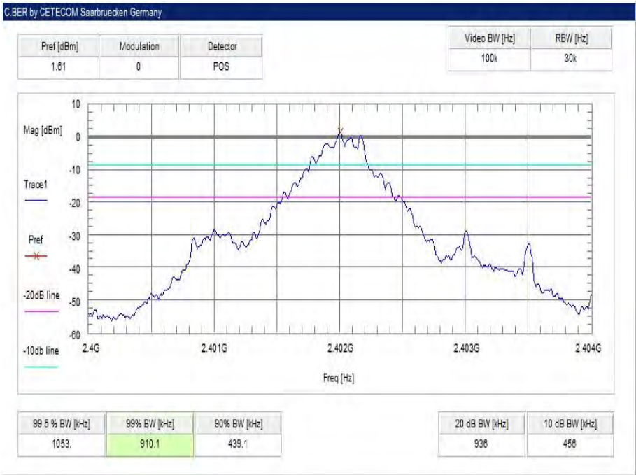
Plot 1: lowest channel – 2402 MHz, GFSK modulation
