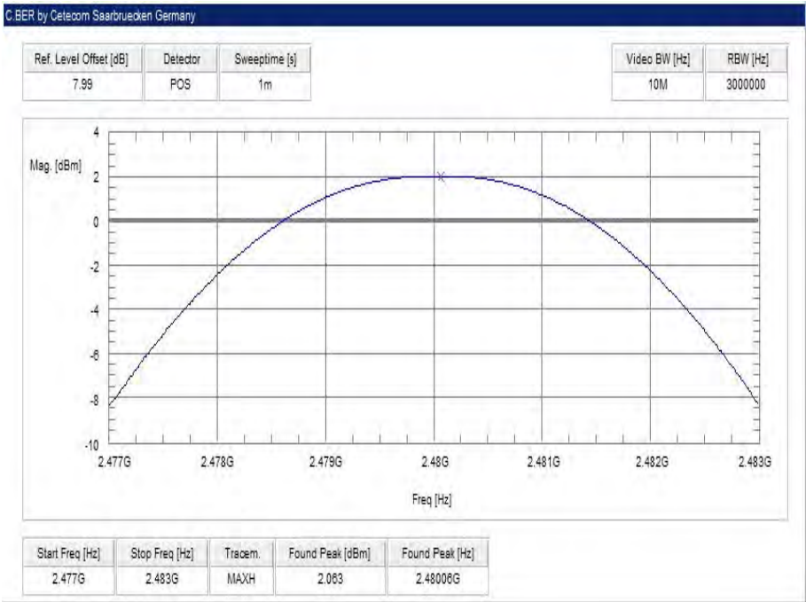
Plot 3: highest channel – 2480 MHz, GFSK modulation
