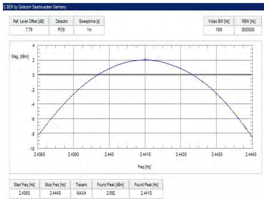
Plot 8: middle channel – 2441 MHz, 8 DPSK modulation
