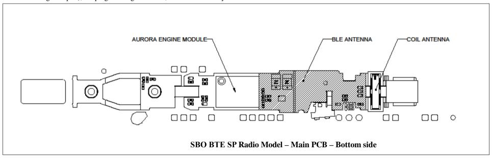
The most important parts inside the Engine module are a Digital-Signal-Processor (DSP), a radio Front-End (FE) chip for the 3.84 MHz radio part and an RF chip for the Bluetooth radio part – all mounted on a small rigid PCB again mounted on the main flex PCB. The SBO BTE SP radio model also includes all voltage regulators and buffered data programming inputs on board. The DSP is the main processor controlling the functionality of both radios in the SBO BTE SP radio model.
