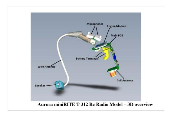
The radio model is implemented in an engine module mounted on the main PCB with connections to the antennas, the microphones, the speaker and the battery terminals. The radio model can be seen in 3D overview to the left:
