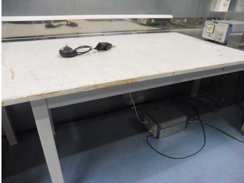
Photo 9: AC conducted test setup
