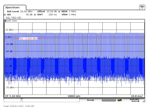
Duty cycle in 100 ms: Burst length \* Number of bursts = 0.212 ms\*160 = 33.9%
