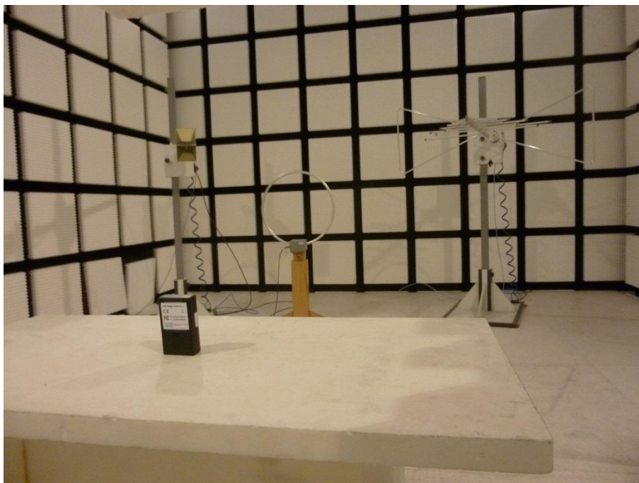
Photo 2: EUT at the anechoic chamber, loop antenna test setup
