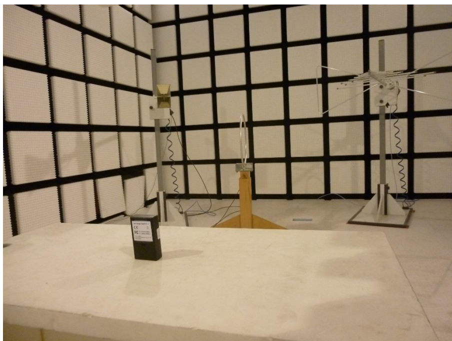
Photo 6: EUT at the anechoic chamber, loop antenna test setup
