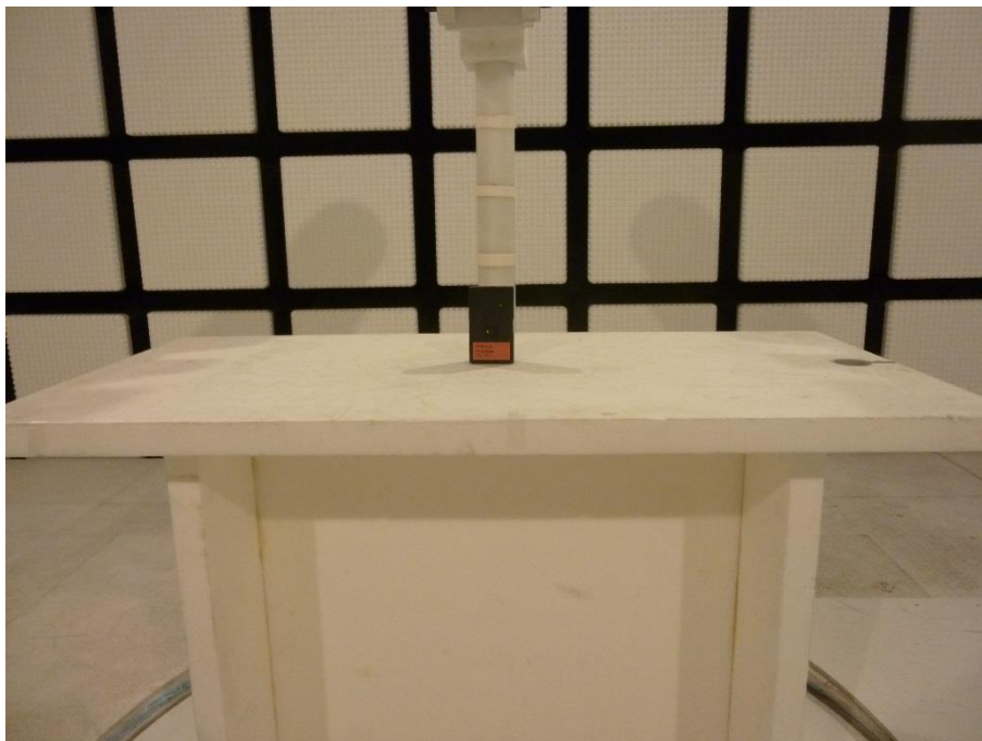
Photo 3: EUT at the anechoic chamber, loop antenna test setup
