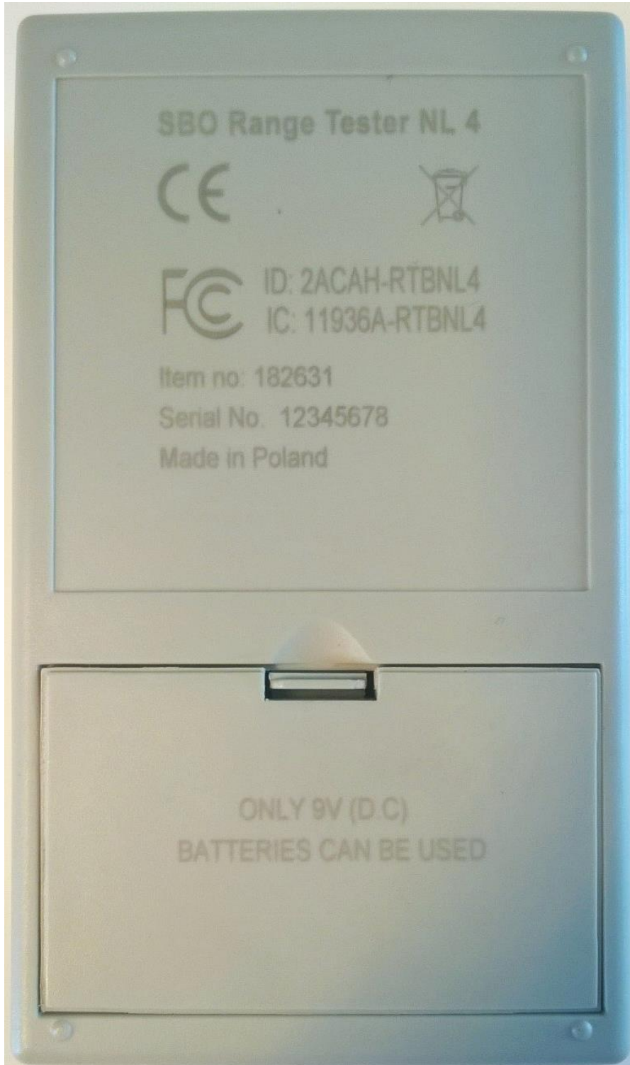
Figure 5. Back side with Type Approval label and battery compartment.
