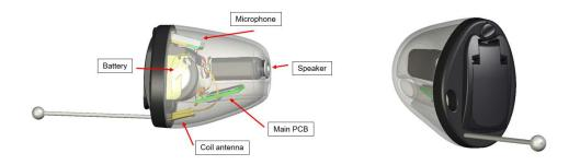
The Aurora CIC radio model is intended to be installed in Philips wireless CIC hearing aid devices (Completely-In-the-Canal) styles.
