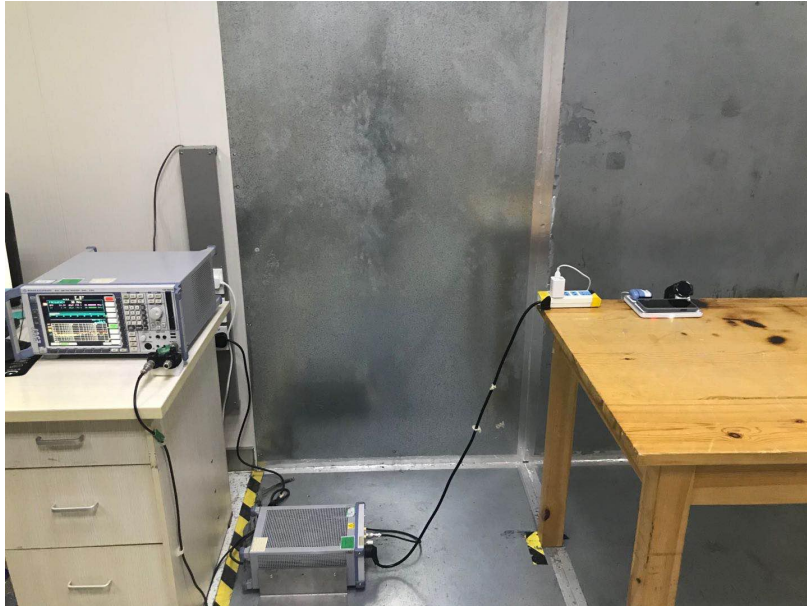
Conducted Emissions Model: 51193
