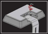
1 Assemble headphones rest to base with included screws and tool. Do not over tighten.
