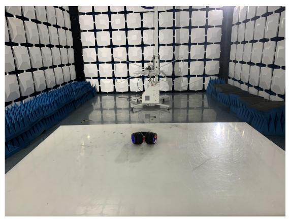
Above 1GHz for radiated emission test setup
