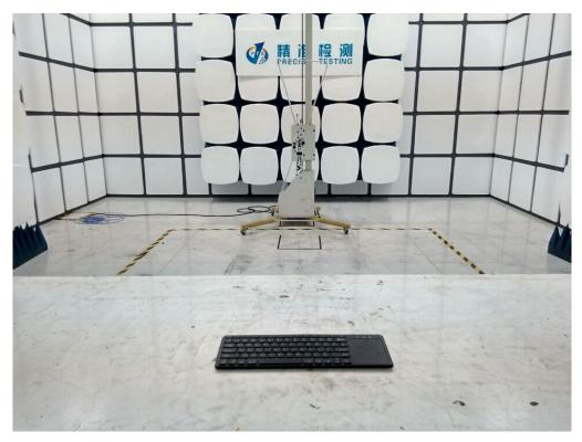
RADIATED EMISSION TEST SETUP ABOVE 1GHz
