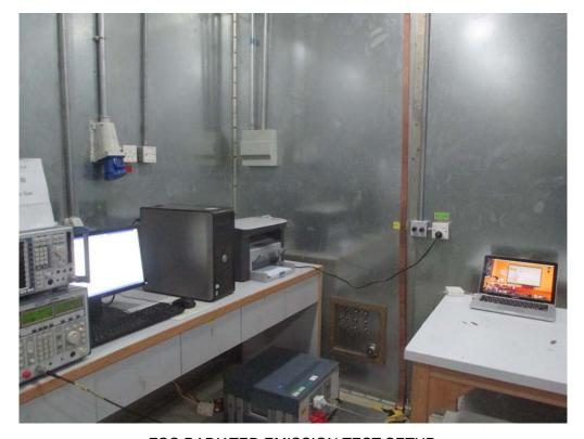
FCC RADIATED EMISSION TEST SETUP
