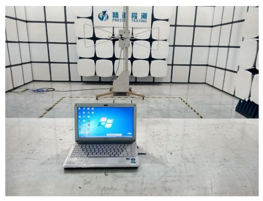
RADIATED EMISSION TEST SETUP ABOVE 1GHz
