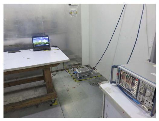
FCC RADIATED EMISSION TEST SETUP
